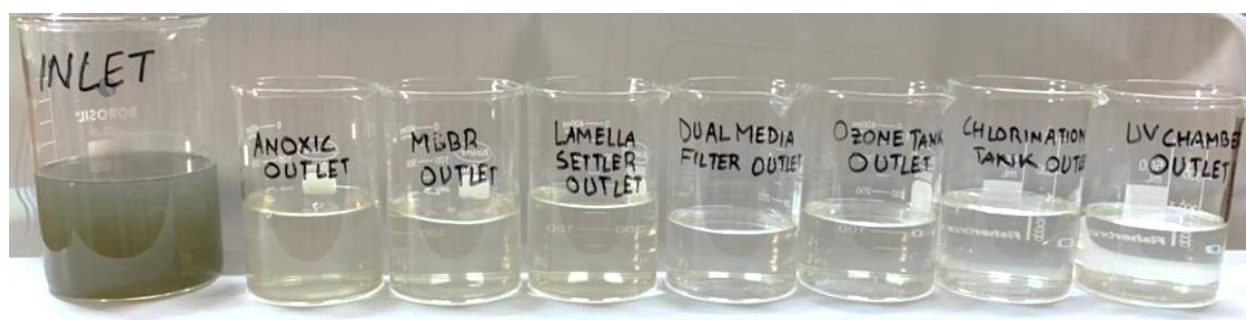
Picture 1: Raw water (left most) and stage wise treated water quality
